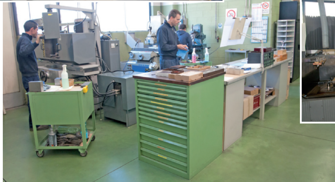
The mechanical tooling department is equipped with several machine tools: horizontal spindle grinding machines, NC milling machines, sinking and wire EDM machines, lathes and machining centres. Here are some of these machines at work.
