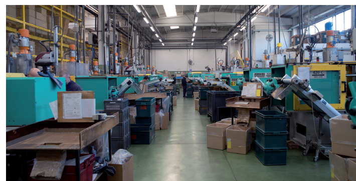
Overview of the moulding department, equipped with 21 Arburg presses for thermoplastic material and three Babyplast for minimum batches and pilot moulds.
